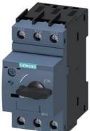
Circuit breaker size S0 for motor protection, CLASS 10 A-release 4.5...6.3 A N-release 82 A screw terminal Standard switching capacity
